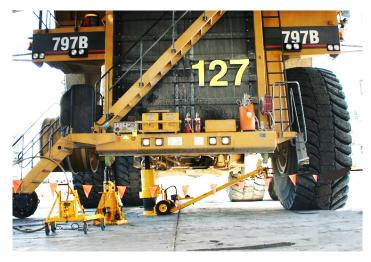
The EDMO AS1 Adjustable Support Stands are designed for supporting vehicles during maintenance and repairs.
